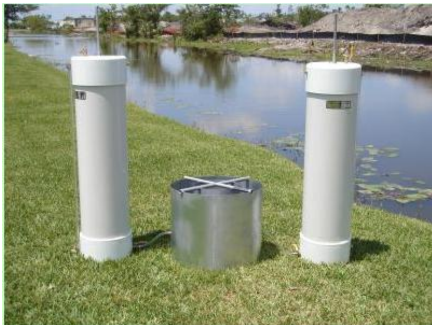
Figure VII.10. Double Ring Infiltrometer Set-up with Mariotte Tubes
