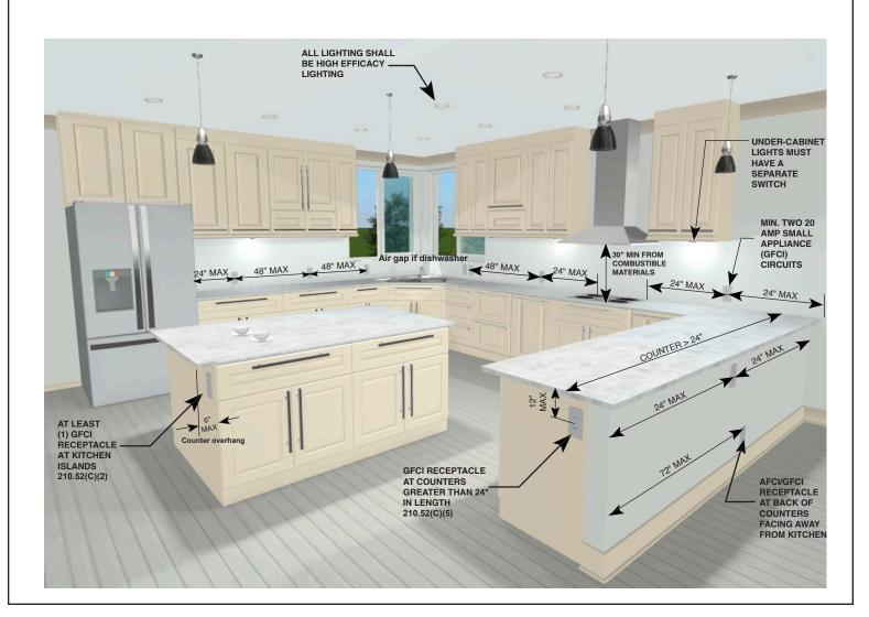
Minimum of two 20-Amp small appliance branch circuits shall be provided to serve all wall & floor receptacles, and counter-top receptacles.[210.11(C)(1)]
