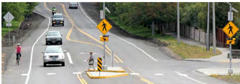
FIGURE 30: EXAMPLE OF ENHANCED PEDESTRIAN CROSSING
