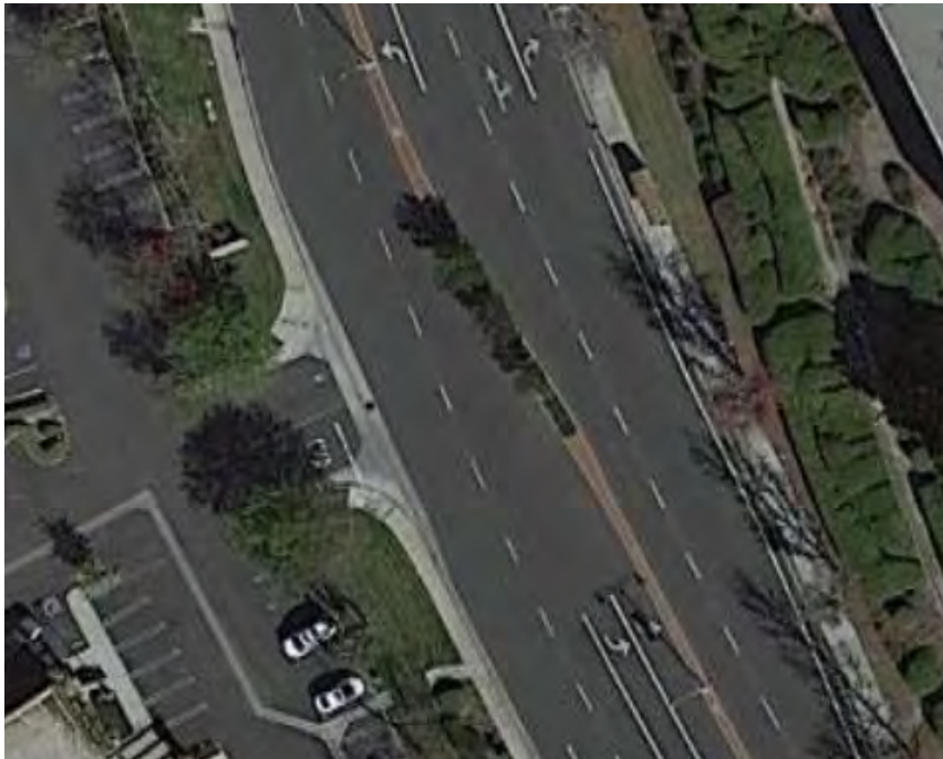
FIGURE 23: EXAMPLE OF CROSS-MEDIAN ACCESS RESTRICTIONS
