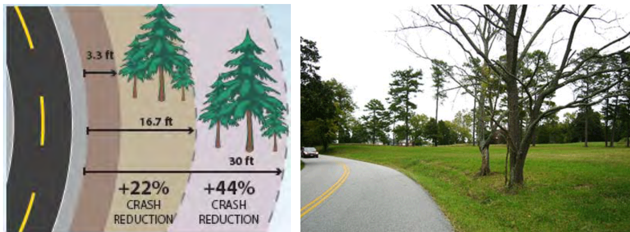
FIGURE 28: EXAMPLE OF REMOVING OR RELOCATING FIXED OBJECT
