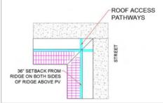
PV More Than 33% Roof Area - Driveway Access (66% for homes with sprinkler systems) [IRC R324.6.1]
