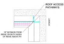
PV Less Than 33% Roof Area - Driveway Access (66% for homes with sprinkler systems) [IRC R324.6.1]
