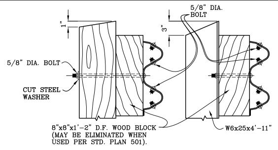
NOTE: SET STEEL RAIL POST IN 9" DIA. HOLE & FILL WITH CONCRETE.
